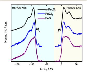
Fig. 2 HEROS-XES to HEROS-XAS transition according to egn (1) for all studied references performed on spectra recorded at an incident energy of 7100 eV.
