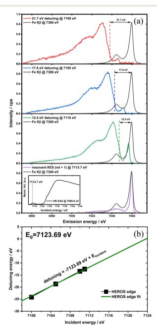
Fig. 3 (a) Detuning parameter  $\delta E$  in the function of incident energy and position changes of HEROS spectra with respect to nXES for FeCl3. The inset shows an incident energy of 7113.7 eV on the HR-XAS spectrum (@7059.6 eV) for which a resonant-XES spectrum was collected; (b)  $\delta E(E_{inc})$  relation with extrapolation to  $\delta E=0$ .
