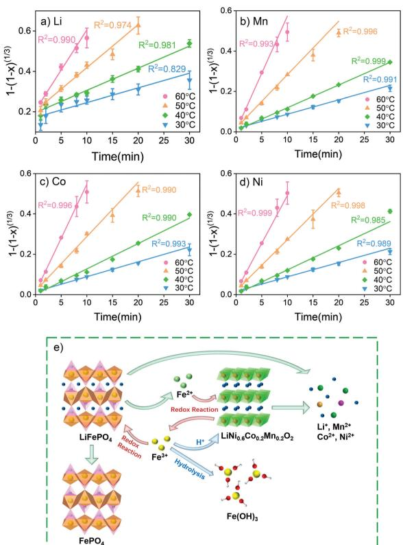
Fig. 3 (a) Fitting results of (a) Li, (b) Mn, (c) Co and (d) Ni, according to a surface chemical reaction model, and (e) reaction mechanisms of synergistic metal extraction from NCM and LFP using Fe<sup>3+</sup> as an intermediate.
