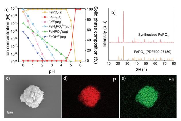
Fig. 4 (a) Calculated ion concentrations and solid phase compositions of  $Fe(III)-PO_4^{3-}$  at different pH values; (b) XRD pattern and (c) SEM image of synthesized  $FePO_4$  after 600 °C calcination; EDX mapping images of (d) P and (e) Fe from synthesized  $FePO_4$  after 600 °C calcination.
