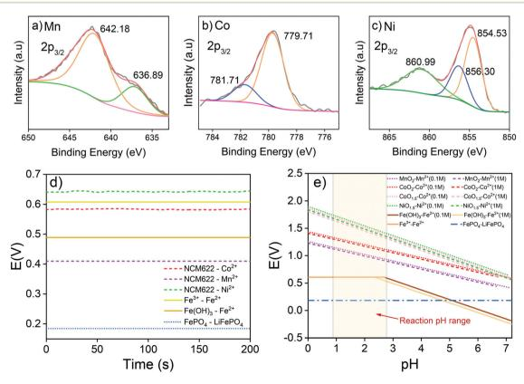
Fig. 1 XPS spectra of (a) Mn, (b) Co, and (c) Ni from the spent NCM622 cathode material; (d) reaction potentials of redox couples; and (e) calculated reaction potentials of redox couples at different pH values according to the Nernst equation.
