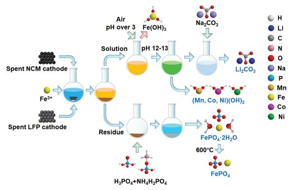
Scheme 1 Flow process for recycling of valuable components in NCM and LFP with Fe<sup>3+</sup> as an intermediate.
