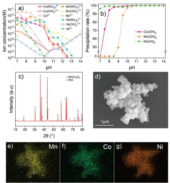
Fig. 5 (a) Calculated ion concentrations of Mn(II), Co(II), and Ni(II) at different pH values. (b) Precipitation rate of  $Mn(OH)_2$ ,  $Co(OH)_2$ , and  $Ni(OH)_2$  at different pH values. (c) XRD pattern and (d) SEM image of the synthesized MnCoNi oxide after 900 °C calcination. EDX mapping image of (e) Mn, (f) Co, and (g) Ni from the synthesized MnCoNi oxide after 900 °C calcination.
