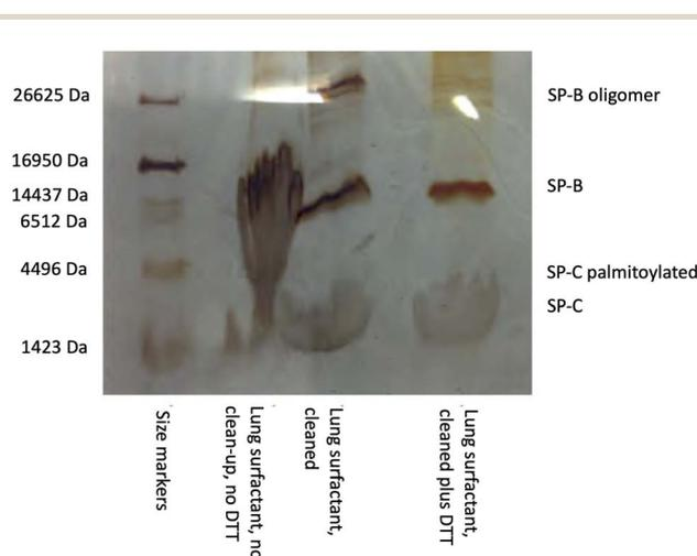
Fig. 1 SDS-PAGE gel with tricine buffer system and silver staining showing the presence of the lung surfactant proteins SP-B and SP-C in extracted porcine lung surfactant. The use of the SDS-PAGE clean-up kit to remove lipids, and the reductant DTT (dithiothreitol), before electrophoresis greatly improved the appearance of the bands, the process also removes the palmitoyl groups from the SP-C protein.
