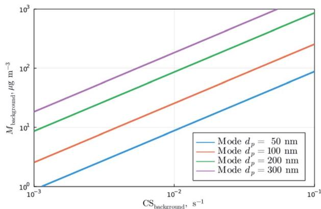
Fig. 8 Mass concentration of background aerosols as a function of their corresponding CS and mode diameter. The other model inputs are:  $\sigma_{\text{geo}} = 1.7$  and  $\rho = 1400 \text{ kg m}^{-3}$ .
