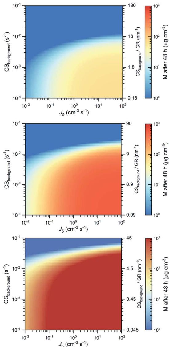
Fig. 7 Mass of the growing mode after 48 h as function of  $J_5$  and  $CS_{\text{background}}$ . The other model inputs are: initial  $d_p = 5$  nm, duration of NPF = 5 h,  $\sigma_{\text{geo}} = 1.7$ , and GR is equal to  $2 \text{ nm h}^{-1}$  (upper panel),  $4 \text{ nm h}^{-1}$  (middle panel) or  $8 \text{ nm h}^{-1}$  (bottom panel).
