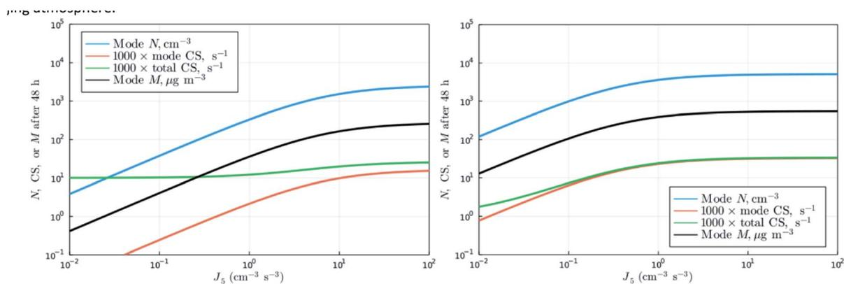
Fig. 5 Number, surface area and mass concentration of the growing mode after 48 h as function of the formation rate of 5 nm particles,  $J_5$ . The condensation sink of the background particle population,  $CS_{\text{background}}$ , has been assumed to be equal to  $0.010 \text{ s}^{-1}$  (left panel) or  $0.001 \text{ s}^{-1}$  (right panel). The other model inputs are: initial particle diameter = 5 nm, duration of NPF = 5 h, GR =  $4 \text{ nm h}^{-1}$  and  $\sigma_{\text{geo}} = 1.7$ .
