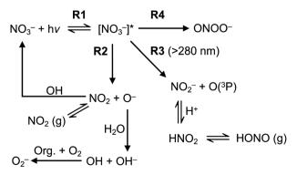
Fig. 1 Simplified nitrate photolysis mechanisms.<sup>50</sup>
