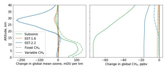
Fig. 6 Change in global mean ozone column (left) and global methane mixing ratios (right) as a result of emissions from each aircraft fleet. Simulations in which the surface methane mixing ratio is fixed are shown with dash-dotted lines ("Fixed CH<sub>4</sub>). Simulations in which surface methane fluxes are prescribed are shown with solid lines ("Variable CH<sub>4</sub>").
