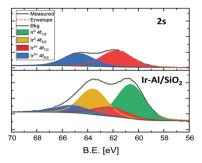
Fig. 3 XPS Ir 4f spectra of materials 2-s (top) and Ir-Al/SiO<sub>2</sub> (bottom)
