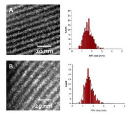
Fig. 2 STEM-HAADF micrographs and Nps size distribution of Ir-Al/SiO<sub>2</sub> (A) and Ir/SiO<sub>2</sub> (B) materials (bar scales: 20 nm).
