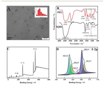
**Fig. 1** (A) HR-TEM images of the pure SQDs with the diameter distribution of the SQDs (inset). (B) FT-IR spectra of the SQDs and pure PEG-400. (C) XPS spectra of the SQDs and (D) the S 2p region.
