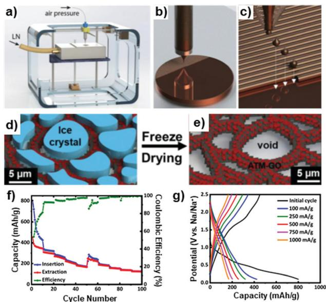
**Fig. 9** (a) Schematics of the 3D “drop-on-demand” ink jet printing setup. (b and c) Printing process of the ATM-GO droplets in a raster fashion. (d) Ice template formation during printing. (e) Resulting ATM-GO aerogel after freeze drying. (f) Rate performance at 5 different current density values. (g) Galvanostatic charge-discharge curves of the first cycle in comparison with those in the 10th cycle. Reproduced with permission.<sup>92</sup> Copyright 2019, Elsevier.
