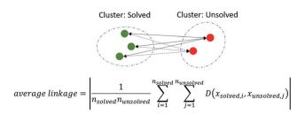
Fig. 2 Illustrates the computation of the average linkage. The average linkage is a method by which the distance between two clusters are treated as the average distance between all pairs of items, where one member of the pair belongs to each cluster.
