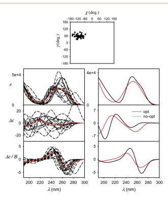
Fig. 5 Spectra of G simulated for ten MD snapshots (dashed) close to minimum I and a 50-snapshot average (solid, red, B3LYP/6-311++G\*\*/CPCM) (left). Averages obtained with and without partial optimization are compared on the right, the geometries are indicated in the  $\chi$ ,  $\gamma$  plane at the top.
