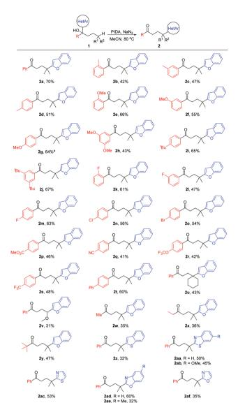
Scheme 2 Substrate scope. Reaction conditions: 1 (0.2 mmol), PIDA (4.0 equiv.), and NaN3 (4.0 equiv.) in MeCN (2.5 mL), 80 °C for 12 h. Yields of the isolated products are given. <sup>a</sup>PIDA (6.0 equiv.) and NaN<sub>3</sub> (6.0 equiv.).
