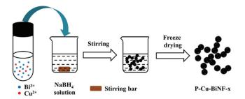
Fig. 1 Schematic diagram of the synthesis of P-Cu-BiNF.
