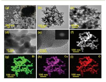
Fig. 2 (a) SEM, (b-d) TEM, (e) HRTEM and (f) HAADF-STEM images and (g-i) TEM-mapping images of P-Cu-BiNF. Insets in (a) and (e) are the optical photo and SAED image of P-Cu-BiNF, respectively.
