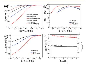
Fig. 4  $\rm CO_2RR$  performances of P-Cu-BiNF, P-Bi and bulk Bi measured in 0.5 M KHCO<sub>3</sub> electrolyte. (a) LSV curves collected under Ar or CO<sub>2</sub> atmosphere at a scan rate of 10 mV s<sup>-1</sup>; potential-dependent (b) FE<sub>formate</sub> and (c)  $j_{formate}$ ; (d) long-term stability test of P-Cu-BiNF at -0.88 V for 12 h.
