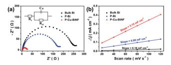
Fig. 5 (a) Electrochemical impedance plots and (b) capacitive  $\Delta i$  (= $i_a$  – j<sub>c</sub>) against scan rate for P-Cu-BiNF, P-Bi and bulk Bi.
