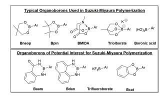
**Fig. 4** Selection of organoborons for cross-coupling. The top group of derivatives have been employed in Suzuki–Miyaura polymerization and the bottom group should be of interest for polymerization. Unsubstituted six-membered boronic esters have also been used as the coupling partner in SM CTP.<sup>51</sup>
