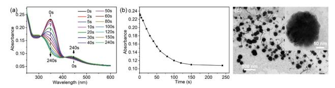
Fig. 3 Disassembly of SKSP nanofibers. (a) UV-vis absorption spectra of the aqueous solution of SKSP nanofibers at different UV irradiation times (365 nm, 250 W). (b) Absorbance at  $\lambda = 350$  nm (*trans*-AZO) as a function of the UV irradiation time. (c) TEM image of the intermediates.
