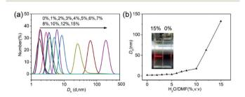
Fig. 1 Complexation and self-assembly of SKSPs. (a) DLS curves of CD-g-HPG-AZOs at various contents of H<sub>2</sub>O in DMF. (b) Dependence of  $D_h$  on the water content for CD-g-HPG-AZOs.
