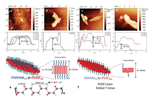
Fig. 9 AFM images of 2D lenticular aggregates prepared from: (a) PNIPAM35-b-PVDF60, (b) PNIPAM35-b-PVDF100, (c) PNIPAM35-b-PVDF150, and (d) PNIPAM35-b-PVDF450. (e and f) Schematic representation and suggested molecular arrangement of the 2D lenticular aggregates formed by the assembly of PNIPAM<sub>35</sub>-b-PVDF<sub>60</sub> and PNIPAM<sub>35</sub>-b-PVDF<sub>450</sub> respectively.
