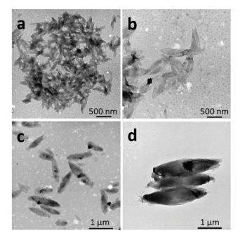
Fig. 6 TEM images of representative self-assembled 2D lenticular morphologies prepared from (a) PNIPAM $_{35}$ -b-PVDF $_{60}$ , (b) PNIPAM $_{35}$ -b-PVDF $_{100}$ , (c) PNIPAM $_{35}$ -b-PVDF $_{150}$  and (d) PNIPAM $_{35}$ -b-PVDF $_{450}$ . All samples were prepared via the solvent switch in acetone: water mixtures. Initial polymer concentration in acetone = 2 mg mL $^{-1}$ . Final concentration = 0.4 mg mL $^{-1}$  in the acetone: water (1:4) mixture. Water addition rate = 4 mL h $^{-1}$ .
