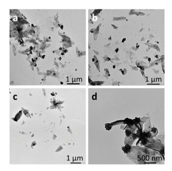
Fig. 10 TEM images of the representative samples of 2D lenticular aggregates prepared from: (a and b) PNIPAM $_{35}$ -b-PVDF $_{150}$  BCPs and (c and d) PNIPAM $_{35}$ -b-PVDF $_{450}$  BCPs in pure water after being heated at 45 °C for 30 min.
