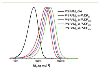
Fig. 1 Normalized SEC traces (viscometric detector) of: PNIPAM $_{35}$ -XA (black trace), PNIPAM $_{35}$ -b-PVDF $_{60}$  (red trace), PNIPAM $_{35}$ -b-PVDF $_{100}$  (blue trace), PNIPAM $_{35}$ -b-PVDF150 (pink trace) and PNIPAM $_{35}$ -b-PVDF450 (green trace) after purification by precipitation in chilled ether for PNIPAM or cold pentane for the BCPs.
