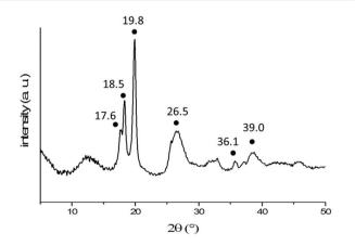
Fig. 8 X-Ray diffraction pattern of freeze-dried 2D lenticular aggregates obtained from PNIPAM<sub>35</sub>-b-PVDF<sub>100</sub> BCPs. The black dots indicate the characteristic peaks of the  $\alpha$ -phase of PVDF.
