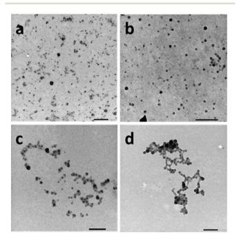
Fig. 2 TEM images of spherical aggregates prepared from (a) PNIPAM $_{35}$ -b-PVDF $_{60}$ , (b) PNIPAM $_{35}$ -b-PVDF $_{100}$ , (c) PNIPAM $_{35}$ -b-PVDF $_{150}$  and (d) PNIPAM $_{35}$ -b-PVDF $_{450}$ . All samples were prepared by nanoprecipitation in water from BCP solutions in DMF at 2 mg mL $^{-1}$  (final concentration = 0.1 mg mL $^{-1}$  in DMF: water (1:20)). Scale bars correspond to 200 nm.
