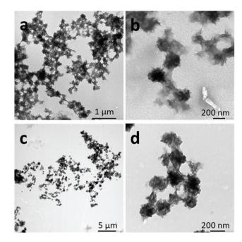
**Fig. 3** TEM images of crumpled aggregates obtained by the solvent switch of (a and b) PNIPAM $_{25}$ -b-PVDF $_{35}$  and (b and c) PNIPAM $_{35}$ -b-PVDF $_{450}$  in DMF at 2 mg mL $^{-1}$ . Final concentration = 0.4 mg mL $^{-1}$  in the DMF : water (1 : 4) mixture.
