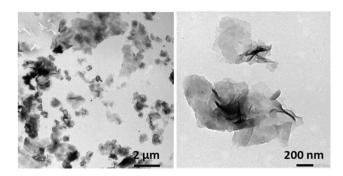
Fig. 4 TEM images of the bilayer aggregates obtained by the solvent switch of PNIPAM $_{35}$ -b-PVDF $_{450}$ . Initial polymer concentration in THF = 2 mg mL $^{-1}$ . Final concentration = 0.4 mg mL $^{-1}$  in the THF: water (1:4) mixture. The water addition rate was 4 mL h $^{-1}$ .
