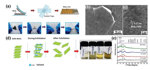
**Fig. 2** (a) Schematic diagram showing the mechanical exfoliation technique for the synthesis of  $MoS_2$  nanosheets, and (b) SEM and (c) HRTEM images of  $MoS_2$  nanosheets. Reproduced from ref. 78 (d) Scheme of the synthesis process *via* the liquid-phase exfoliation of  $MoS_2$  nanosheets and (e) X-ray diffraction patterns of bulk  $MoS_2$  powder and  $MoS_2$  nanosheets synthesized using different initial concentrations of bulk  $MoS_2$ . Reproduced from ref. 81.
