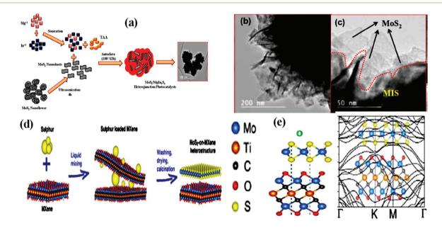
Fig. 6 (a) Schematic diagram showing the growth mechanism and (b) and (c) corresponding HRTEM images of  $MoS_2/MgIn_2S_4$  heterojunction photocatalyst. Reproduced with permission.<sup>90</sup> (d) Schematic representation of the fabrication of  $MoS_2/MX$ ene hybrids and (e) structural stacking patterns and electronic band structure of  $MoS_2/Mo_2TiC_2O_2$ . Reproduced with permission.<sup>105</sup>
