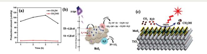
Fig. 14 (a) Rate of  $CO_2$  reduction by  $MoS_2$  sheets in 0.5 M NaHCO<sub>3</sub> and (b) schematic representation of the mechanistic pathway for photocatalytic  $CO_2$  reduction over  $MoS_2$  sheets. Reproduced with permission.<sup>173</sup> (c) Schematic illustration of the photoreduction of  $CO_2$  to  $CH_3OH$  in the  $MoS_2/TiO_2$  heterostructure. Reproduced with permission.<sup>170</sup>
