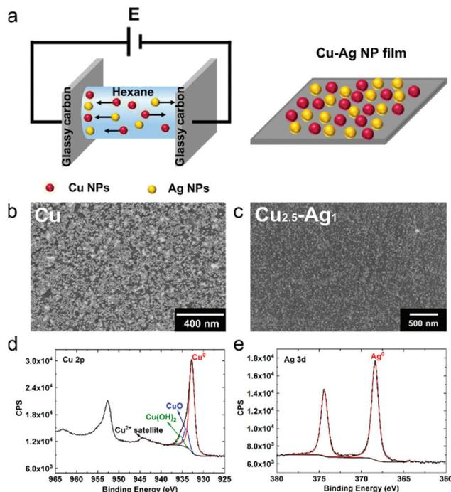
**Fig. 3** (a) Schematic illustration of the film preparation *via* electrophoresis. The arrows indicate the moving direction of NPs under applied potential. (b and c) SEM images of the anode Cu (b) and  $\text{Cu}_{2.5}\text{-Ag}_1$  (c) NPs film prepared at 100 V for 60 min. (d and e) Cu 2p (d) and Ag 3d (e) XPS spectra of a  $\text{Cu}_{2.5}\text{-Ag}_1$  NPs film prepared by electrophoresis at 100 V for 60 min.
