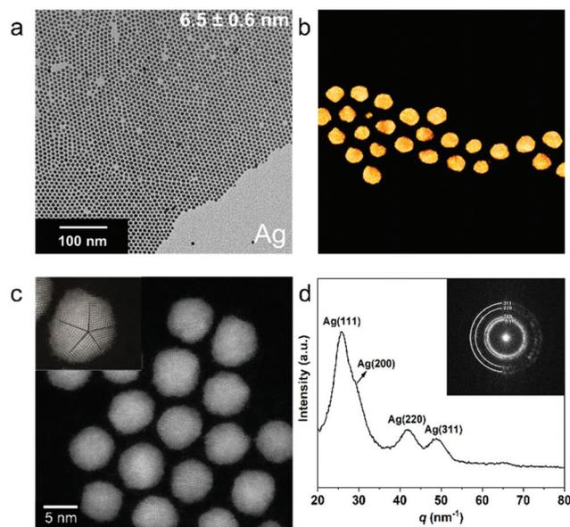
**Fig. 2** (a) TEM image of colloidal Ag NPs. (b) 3D visualization of the reconstructed volume of a number of Ag NPs. (c) High resolution HAADF-STEM image of Ag NPs, showing the polycrystallinity of the NPs and the presence of pentatwinned domains. A magnified image of a region with a pentatwinned domain is shown as inset. (d) Fourier transform (FT) pattern (inset) of Ag NPs and the radially integrated 1D Powder Electron Diffraction (PED) pattern.
