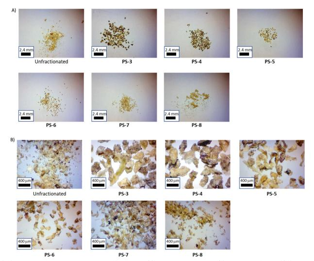
Optical micrographs demonstrating the range of particle sizes (A) and irregular particle shapes (B) in peanut shell fractions PS-X.
