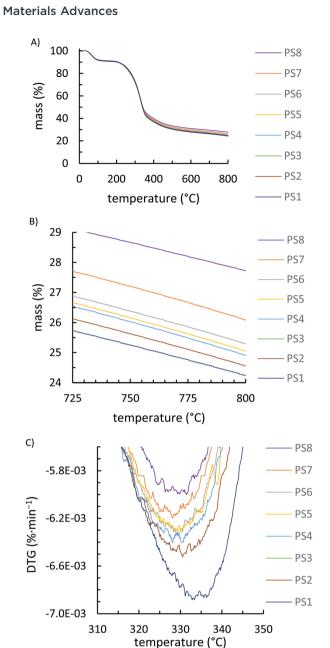
Fig. 3 Thermogravimetric analysis of **PS-X** fractions from 25–800 °C (A), from 725-800 °C to emphasize the difference in residual mass (B), and the derivative TGA (DTG) curve over the primary decomposition step, emphasizing the more rapid and lower-temperature decomposition with smaller particle size (C). Note that PS-2 and PS-3 are coincident.
