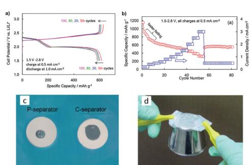
Fig. 14 (a) Voltage profile in selected cycles and (b) rate capability of the Li/S cell with the C-separator. (c) Wettability of the liquid electrolyte on separator and (d) gluing ability of the C-separator immediately after being wetted with a liquid electrolyte. Image reprinted with the permission from ref. 106. Copyright © 2013, Elsevier License 5041390032620.
