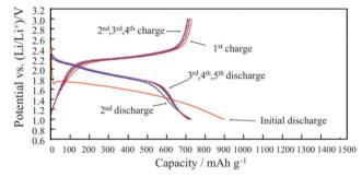
Fig. 2 Charge/discharge performance of SPAN cathode in 1 M LiPF<sub>6</sub>/EC + DEC. Image reprinted with the permission from ref. 49. Copyright © 2012, Elsevier License 5041181200155
