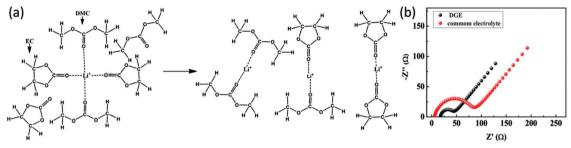
Fig. 3 (a) Schematic diagram of the solvation of Li ions in common electrolyte and concentrated desolvated gel electrolyte (DGE) and (b) impedance plots of Li–S cells with DGE and common electrolyte after the third cycle. Image reprinted with the permission from ref. 50. Copyright © 2014, American Chemical Society.
