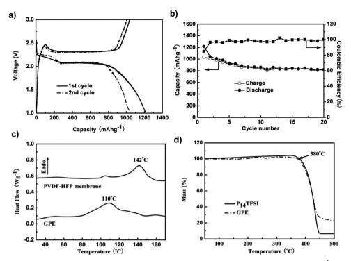
Fig. 12 (a) Charge-discharge curves and (b) cycling performance of the Li/GPE/S battery at a current density of 50 mA  $g^{-1}$ . (c) DSC curves of P(VDF-HFP) membrane and GPE, and (d) TGA of P14TFSI and GPE. Image reprinted with the permission from ref. 104. Copyright © 2012 Elsevier License 5041380226718
