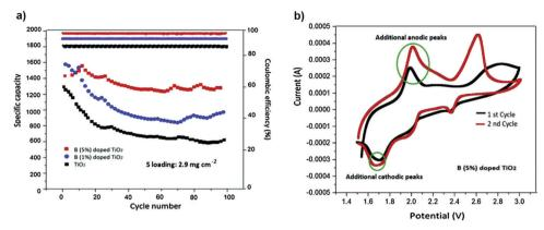
Fig. 26 (a) Cycling performance and coulombic efficiency of Li-S cells for three different coatings at 1 C. (b) First two CV curves of the cell with a 5% Bdoped TiO<sub>2</sub> coating swept at 0.1 mV s<sup>-1</sup>. Image reprinted with the permission from ref. 140. Copyright © 2020, Elsevier License 5040720744337.
