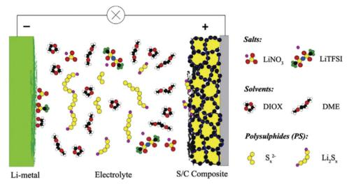
Fig. 1 Schematic of the components of a state-of-the-art Li/S battery with an electrolyte consisting of LiTFSI in a 1:1 mixture of DME and DIOX. Image reprinted with the permission from ref. 29. Copyright © 2014, Elsevier License-5041171085878.
