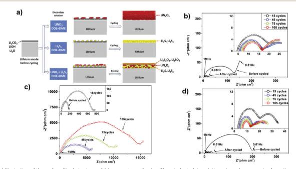
Fig. 27 (a) Illustration of the surface film behavior on lithium anode cycling in different electrolyte solutions. Impedance spectra from the symmetrical cells containing (b) 0.2 M Li<sub>2</sub>S<sub>6</sub>/DIOX/DME, (c) 0.2 M LiNO<sub>3</sub>/DIOX/DME and (d) 0.1 M LiNO<sub>3</sub>/0.1 M Li<sub>2</sub>S<sub>6</sub>/DIOX/DME. Image reprinted with the permission from ref. 143. Copyright © 2014, Elsevier License 5041340287373.
