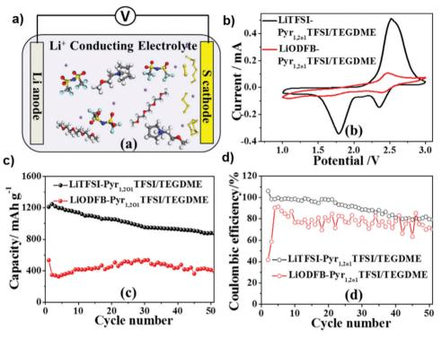
Fig. 23 (a) Schematic illustration of the  $Pyr_{1,2O1}TFSI/TEGDME$  electrolyte with LiTFSI. (b) CVs of the Li-S cells containing the  $Pyr_{1,2O1}TFSI/TEGDME$  electrolytes with LiTFSI and LiODFB. (c) Cycling performance and (d) coulombic efficiency of the Li-S cells with the LiTFSI- $Pyr_{1,2O1}TFSI/TEGDME$  and LiODFB- $Pyr_{1,2O1}TFSI/TEGDME$  electrolytes. Image reprinted with permission from ref. 137. Copyright © 2015, Elsevier License 5041420221520.
