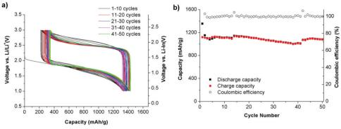
Fig. 20 (a) Discharge-charge curves and (b) discharge/charge capacity and coulombic efficiency of the all-solid-state S/Li<sub>6</sub>PS<sub>5</sub>Br/In-Li cell up to 50 cycles at room temperature. Image reprinted with permission from ref. 134. https://doi.org/10.1007/s10008-014-2654-1.
