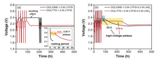
Fig. 30 Voltage profile for Li-S cells rested for an extended period of time with DOL/DME-1.0 M LiTFSI and DOL/TTE-1.0 M LiTFSI (a) without LiNO<sub>3</sub> and (b) with 0.2 M LiNO<sub>3</sub>. Image reprinted with permission from ref. 148. Copyright © 2014, IOP publishing, J. Electrochem. Soc.
