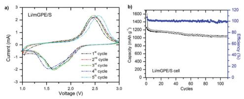
Fig. 13 (a) CV profiles for the Li/mGPE/S cell and (b) charge-discharge versus cycles at a 0.2 C rate. Image reprinted with the permission from ref. 105. Copyright © 2013, Royal Society of Chemistry License 1116861-1.
