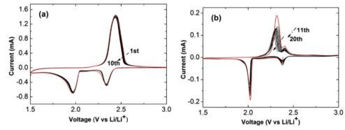
Fig. 9 CV curves of Li-S cells with 1 M LiTFSI in PP13-TFSI/DME (2/1, v/v). (a) The first 10 cycles at 0.1 mV s<sup>-1</sup> and (b) the subsequent 10 cycles. Image reprinted with the permission from ref. 74. Copyright © 2013, Elsevier License 5041360562040
