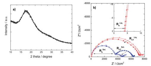
Fig. 19 (a) XRD diffraction pattern of  $\text{Li}_3\text{PS}_4$  and (b) Nyquist plots of solid (blue) and liquid (red) electrolyte symmetrical Li/Li cells at  $-20\,^{\circ}\text{C}$ . Image reprinted with the permission from ref. 133. Copyright © 2015 IOP publishing *J. Electrochem. Soc.* https://doi.org/10.1149/2.0441504jes.
