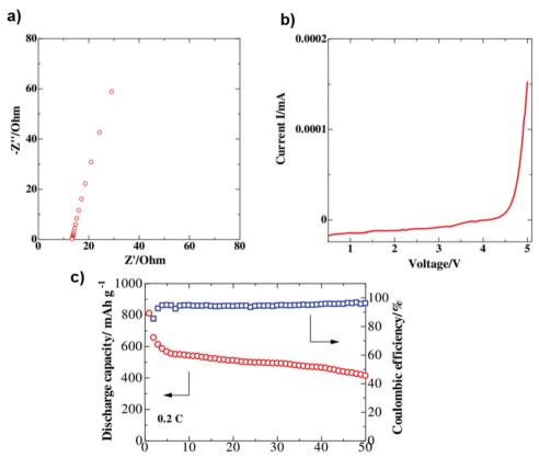
Fig. 15 (a) Impedance spectrum of the as-prepared gel polymer electrolyte. (b) CV profile of the Li/GPE/SS cell (scan rate 0.1 mV s<sup>-1</sup>). (c) Cycling performance of the gel polymer cell with S/GNS composite cathode at 0.2 C. Image reprinted with the permission from ref. 107. https://doi.org/10.1186/1556-276X-9-137.
