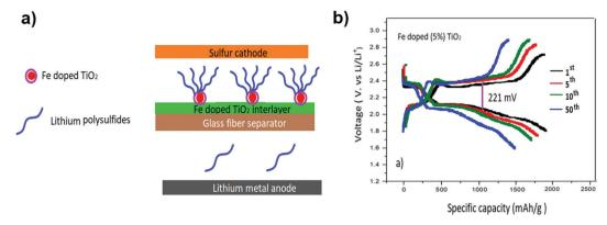
Fig. 28 (a) Schematic for the Li-S battery configuration with the Fe-doped TiO<sub>2</sub> interlayer on a glass fiber separator. (b) Discharge-charge voltage profiles of the Li-S cell with a 5% Fe-doped TiO<sub>2</sub> separator at 1 C. Image reprinted with the permission from ref. 144. Copyright © 2020, Elsevier License 5041340812636
