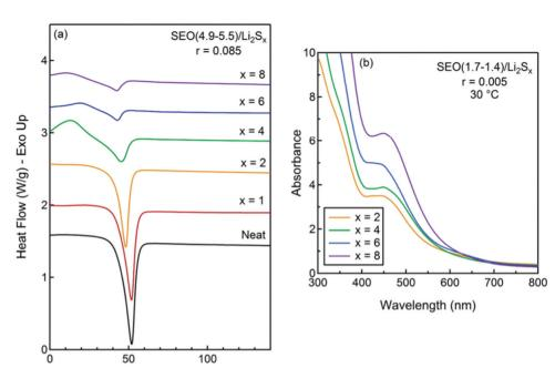
Fig. 11 (a) DSC traces of SEO  $(4.9-5.5)/\text{Li}_2\text{S}_x$  at r = 0.085 and a heating rate of 10 °C min<sup>-1</sup>, and (b) UV-vis spectra of dry mixtures of Li<sub>2</sub>S<sub>x</sub> at r = 0.005 in SEO (1.7-1.4) at 30 °C. Image reprinted with the permission from ref. 103. Copyright © 2011, American Chemical Society.
