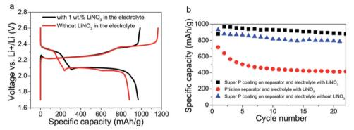
Fig. 25 (a) First charge/discharge voltage profiles of the Li–S batteries using the electrolyte with and without 1 wt% LiNO<sub>3</sub>, respectively. (b) Cycling stability comparison of the Li–S batteries with different separators and electrolytes at C/10. Image reprinted with the permission from ref. 139. Copyright © 2014, Royal Society of Chemistry License 1116742-1.
