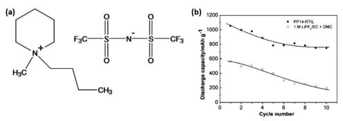
Fig. 6 Comparison of the cycling capacity of Li/S cells in (a) the IL electrolyte and (b) 1 M LiPF<sub>6</sub>/EC + DMC. Image reprinted with the permission from ref. 71. Copyright © 2006, Elsevier License 5041350380913.
