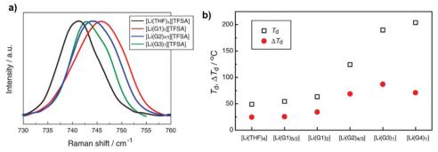
Fig. 7 (a) Raman spectra of [Li(glyme or THF)<sub>x</sub>][TFSA] mixtures. (b) Thermal decomposition temperature ( $T_d$ ) and its difference ( $\Delta T_d$ ) from  $T_d$  of the pure solvents of [Li(glyme or THF)<sub>x</sub>][TFSA] mixtures. Image reprinted with the permission from ref. 72. Copyright © 2013, Elsevier License 5041350752944.
