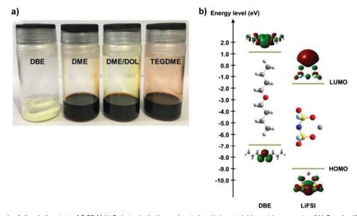
Fig. 4 (a) Photograph of dissolution test of 0.25 M  $\text{Li}_2\text{S}_6$  in typical ether solvents by stirring stoichiometric amounts of  $\text{Li}_2\text{S}$  and sulfur in the solvents for 24 h. (b) The LUMO and HOMO energy values of DBE and LiFSI obtained by DFT simulations. Image reprinted with the permission from ref. 61. Copyright © 2018, Royal Society of Chemistry License-1117493-1.
