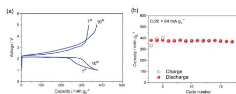
Fig. 18 (a) Voltage profiles and (b) cycling behavior of a Li/Li<sub>2</sub>S−P<sub>2</sub>S<sub>5</sub>/S−MCMB cell. Image reprinted with the permission from ref. 132. Copyright © 2021, Elsevier License 5041400972622.
