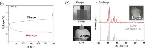
Fig. 10 (a) Prismatic design of electrochemical Li-extraction process. (b) Charge and discharge voltage profile during Li-extraction. (c) Li metal formation after charging and  $\text{Li}_2\text{CO}_3$  formation after discharging.
