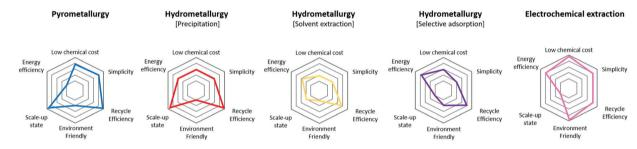
Fig. 11 Performance and industrial comparisons of lithium recycling technologies from waste LIBs, pyrometallurgy, hydrometallurgy and electrochemical extraction.
