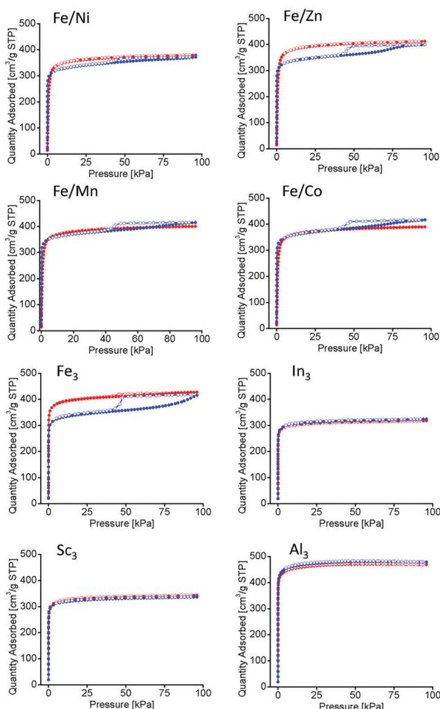
Fig. 5 Nitrogen Isotherms at 77 K before (red) and after (blue) 100 hour thermal activation. In the Fe/Ni, Fe/Zn, Fe/Mn, Fe/Co,  $\text{Fe}_3$ , clusters a hysteresis loop is observable indicating mesopore formation. Samples for  $\text{In}_3$ ,  $\text{Sc}_3$ , and  $\text{Al}_3$  do not have mesopore formation.
