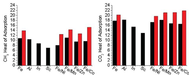
Fig. 6 The average heat of adsorption for  $\text{CH}_4$  and  $\text{CO}_2$  for the microporous (black) and mesoporous (red) sample isomorphs. Heat of adsorption was calculated based on the experimental adsorption isotherms at 195 K, 273 K, and 298 K for each gas.
