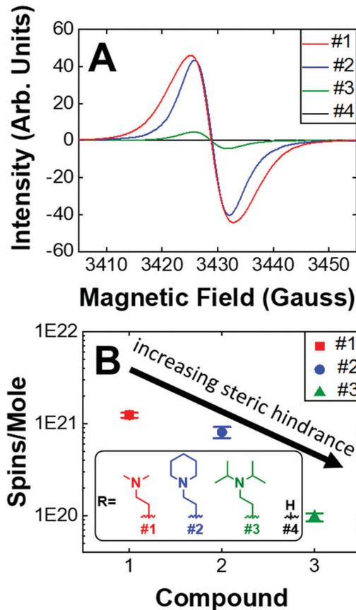
Fig. 5 (A) Raw EPR spectra. Maximum intensities of compounds **1–4**. (B) Average spin concentrations of compounds **#1–3**. Compound **4** is not spin active. (inset) Dopant structures and control compound **#4**.
