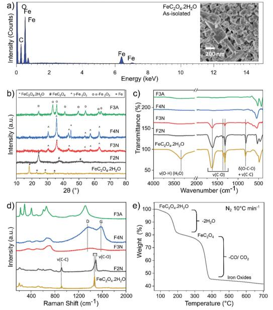
Fig. 1 (a) SEM-EDX spectral data and (inset) SEM image of as-isolated material. (b) PXRD patterns (c) FTIR spectra, (d) Raman spectra of as-isolated and heat-treated FeC<sub>2</sub>O<sub>4</sub>·2H<sub>2</sub>O, revealing chemical and structural changes after heat treatment. (e) Weight loss profile of as-isolated FeC<sub>2</sub>O<sub>4</sub>·2H<sub>2</sub>O during thermal decomposition in N<sub>2</sub> (10 °C min<sup>-1</sup>).
