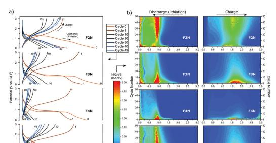
Fig. 6 (a) Potential profiles and (b) differential capacity maps of F2N, F3N, F4N and F3A galvanostatically cycled 50 times at 100 mA  $g^{-1}$ . Differential capacity maps during discharge and charging show the changes to the charge and discharge capacity delivered at each potential as cycling progressed.
