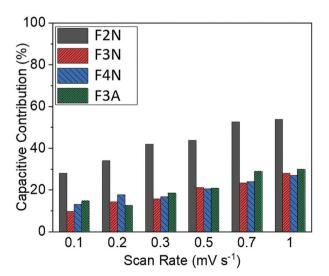
Fig. 5 Capacitive contributions for heat-treated materials at scan rates of 0.1-1 mV s<sup>-1</sup> for F2N, F3N, F4N and F3A
