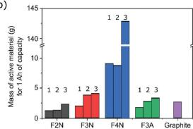
Fig. 7 Carbon content of heat-treated samples. (a) Amount of carbon per gram of heat-treated material before and after heat treatment. (b) Mass of heat-treated material required to store 1 A h of capacity at three scenarios; (1) cycle 220–240, 100 mA  $g^{-1}$ , (2) 50th cycle, 100 mA  $g^{-1}$ , (3) average at 400 mA  $g^{-1}$ . The value for graphite is provided as a reference, and is based on its theoretical capacity.
