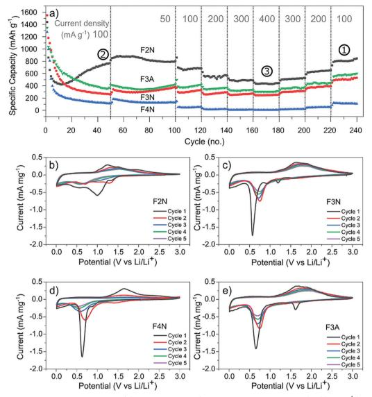
Fig. 4 (a) Discharge capacity of heat-treated samples (F2N, F3N, F4N and F3A) during galvanostatic cycling at 50-400 mA  $g^{-1}$  (relative to the active material mass). Specific capacities used for determining carbon content per Ah (Fig. 7) are indicated by the numbers (1, 2, and 3). (b)–(e) Cyclic voltammograms of (b) F2N, (c) F3N, (d) F4N and (e) F3A between 3.0-0.0 V vs. Li/Li<sup>+</sup> at a scan rate of 0.1 mV s<sup>-1</sup>.
