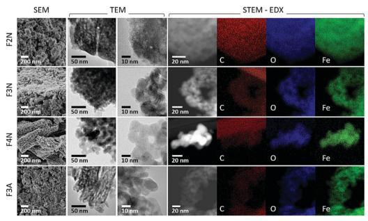
Fig. 3 SEM and TEM images showing the morphology of heat-treated samples (F2N, F3N, F4N and F3A). STEM-EDX elemental maps of  $FeC_2O_4 \cdot 2H_2O_4 \cdot 2H_2O_4$
