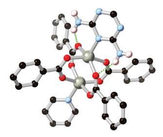
Fig. 8 The heterocycle-capped copper paddlewheel nodes in the MOF of L14 reported by Zhang, showing the hydrogen bonding between the diaminotriazine group and two coordinating carboxylates.<sup>78</sup> The D-A distances are 2.88 and 2.93 Å, and the D-H...A angles are 150 and 138° respectively.
