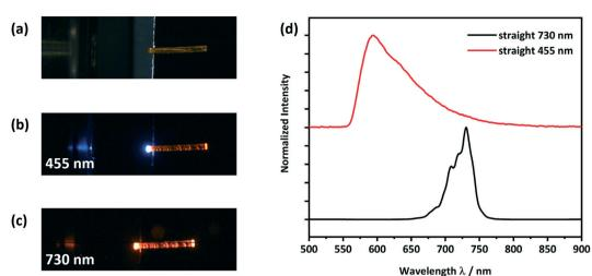
Fig. 7 Optical microscope images of a) a form II straight crystal placed on a silicon wafer with a 3  $\mu$ m thick SiO<sub>2</sub> layer as shown in Scheme S1,† b) showing light with a wavelength of 455 nm being coupled at the left end of the crystal and c) showing light with a wavelength of 730 nm being coupled at the left end of the crystal; d) detected PL spectra at the right end of the crystal. The spectra of the LED light sources, PLE and PL are given in Fig. S11 and S12.†
