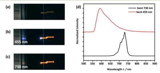
Fig. 8 Optical microscope images of (a) the bent crystal placed on a silicon wafer with a 3  $\mu$ m thick SiO<sub>2</sub> layer, (b) showing light with a wavelength of 455 nm being coupled at the left end of the crystal and (c) showing light with a wavelength of 730 nm being coupled at the left end of the crystal; (d) detected PL-spectra at the right end of the crystal.
