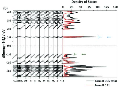
Fig. 6 Selected areas of the band structure and density of states (DOS) of (a) form I and (b) form II. The black line shows the total DOS and the red line represents the DOS projected onto C-based atomic 2pz orbitals. The blue arrow indicates the conduction band and the green arrow indicates the valence band. The complete band structure is provided in the ESI,† Fig. S8 and S9.
