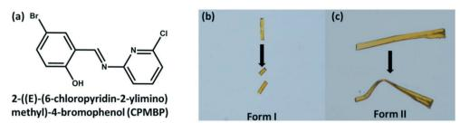
Fig. 1 (a) Chemical structure of the title compound, CPMBP. (b and c) Optical images showing the brittle and plastic deformation behaviour of form I and form II, respectively.
