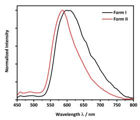
Fig. 5 Solid-state photoluminescence spectra of the brittle (form I. black line) and plastic (form II, red line) forms of CPMBP ( $\lambda_{ex}$  = 425
