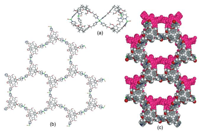
Fig. 8 Crystal structure of  $[Cu_3(L3)_4(H_2O)_3] \cdot 6(OTf) \cdot n(DMSO)$ . (a) Two  $Cu_3L_2$  capsules linked through a shared Cu(n)-vertex; (b) 2D network of linked capsules; (c) packing of two network layers (one in pink) showing substantial channels with largest ca. 1.5 × 3 nm cross-section.<sup>20</sup>
