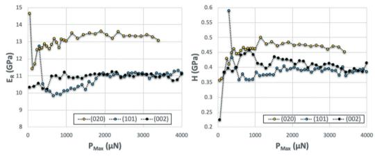
Fig. 6 Series of nanoindentation measurements carried out with increasing P<sub>Max</sub> on three single crystals of CBZ oriented along the three different crystal directions. The derived  $E_R$  (left) and H (right) as a function of  $P_{Max}$  appear fairly constant across the entire range tested.
