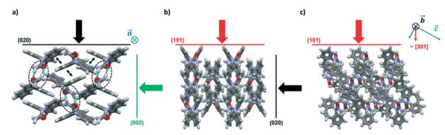
Fig. 3 Packing views of CBZ-III (CBMZPN02) along three directions (a-c) with indentation directions orthogonal to the three main indexed faces indicated as black, green and red arrows. Hydrogen bonded dimers are indicated in (a) with black dashed circles and aromatic interactions via small black double headed arrows.
