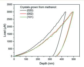
Fig. 4 Load-depth curves from indentation carried out on a (020), a (101) and a (002) face of single crystals of carbamazepine form III crystals.
