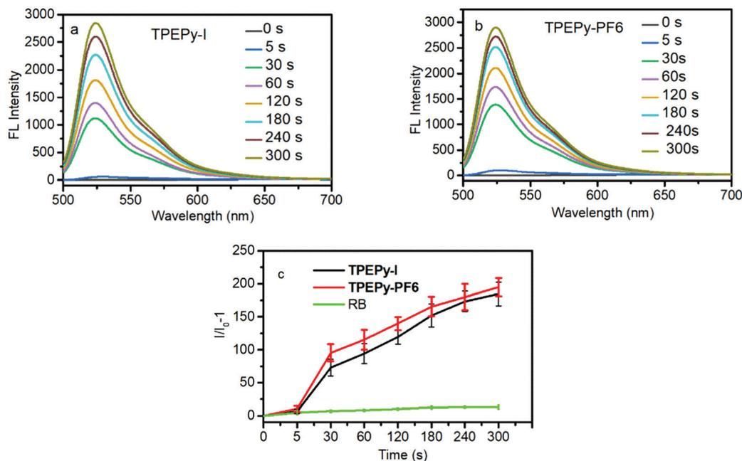
Fig. 1 Change of PL intensity at 525 nm of H<sub>2</sub>DCF-DA in the presence or absence of (a) TPEPy-I (10 μM) and (b) TPEPy-PF6 (10 μM). (c) The fluorescence enhancement ratio of 525 nm of H<sub>2</sub>DCF-DA in the presence of the two AIEgens or RB upon light irradiation for different time durations.
