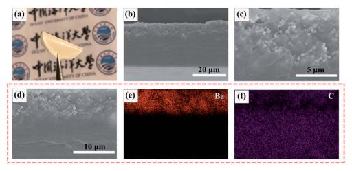
Fig. 2 (a) Photograph, (b-d) cross-sectional SEM morphologies and (e and f) corresponding EDX mapping images of the PEI-20 vol% BT/PVDF bilayer composite.
