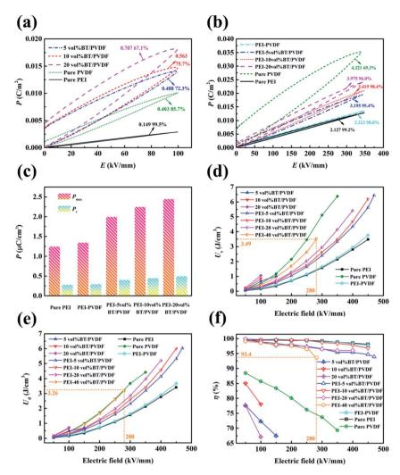
Fig. 5 P-E loops of (a) single layer composites and (b) bilayer composites with different BaTiO<sub>3</sub> loadings. (c) The maximum displacement  $P_{\text{max}}$ and remnant displacement  $P_r$  of the pure PEI and bilayer composites at 350 kV mm<sup>-1</sup>. (d) The storage energy densities, (e) discharge energy densities and (f) discharge efficiencies of the single layer and bilayer composites under varied external electric fields.
