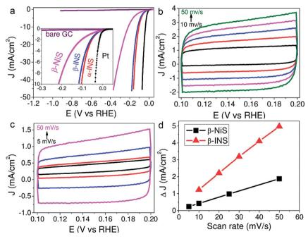
Fig. 5 (a) HER LSVs of  $\beta$ -NiS,  $\beta$ -INS,  $\alpha$ -INS and Pt showing the superiority of INS electrodes over NiS. (b and c) CVs recorded at different scan rates to calculate the relative ECSA of  $\beta$ -NiS and  $\beta$ -INS, respectively. (d) The plot of scan rate against the difference in the double layer charging current density of the same showing higher relative ECSA for  $\beta$ -INS. Reproduced with permission from ref. 64 (Copyright 2015 American Chemical Society).
