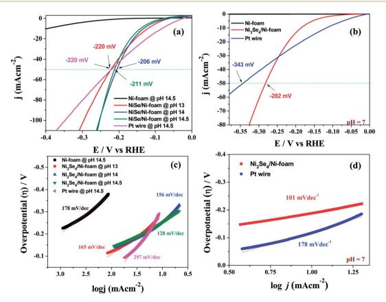
Fig. 9 (a and b) HER LSVs of a Ni<sub>3</sub>Se<sub>4</sub>/Ni electrode in various alkaline pHs and in PBS, respectively. (c and d) The Tafel plots of the same under identical electrochemical conditions. Reproduced with permission from ref. 79 (Copyright 2017 American Chemical Society).
