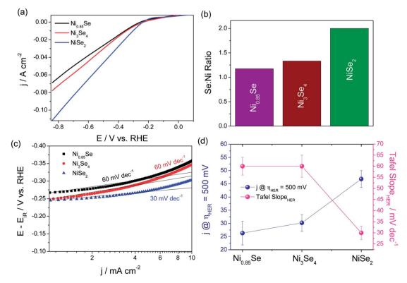
Fig. 10 (a) HER LSVs of  $Ni_{0.85}Se$ ,  $Ni_3Se_4$  and  $NiSe_2$  with identical catalyst loading in 0.5 M  $H_2SO_4$ . (b) Histogram showing the Ni : Se ratio. (c) The Tafel plots of  $Ni_{0.85}Se$ ,  $Ni_3Se_4$  and  $NiSe_2$ . (d) Comparison of activity and kinetics of  $Ni_{0.85}Se$ ,  $Ni_3Se_4$  and  $NiSe_2$  in terms of HER current density at an overpotential of 500 mV and the Tafel slope. Reproduced with permission from ref. 80 (Copyright 2019 Elsevier Publications).
