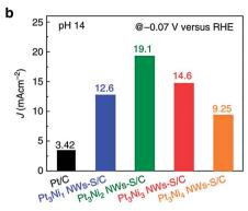
Fig. 6 (a) HER LSVs of compositionally segregated Pt-Ni NWs/NiS heterostructured electrodes in alkali (pH 14) recorded at 10 mV s<sup>-1</sup> with 1600 rpm and presented without iR drop compensation. (b) Histogram showing the current density of the studied catalysts at -0.07 V vs. RHE. Adapted from ref. 67.
