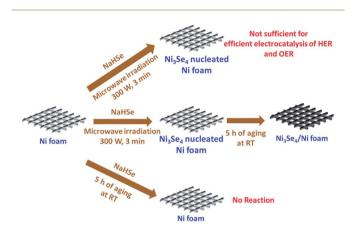
Scheme 2 Synthesis of Ni<sub>3</sub>Se<sub>4</sub> on Ni foam utilizing quick microwave irradiation and room temperature aging. Reproduced with permission from ref. 79 (Copyright 2017 American Chemical Society)
