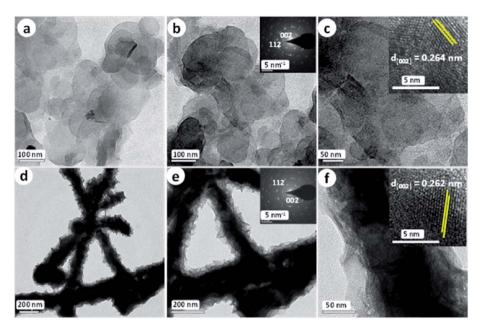
Fig. 11 (a–c) TEM images of NiTe<sub>2</sub> NFs. The insets of (b) and (c) are the respective SAED pattern and HRTEM image. (d–f) TEM images of NiTe<sub>2</sub> NWs. The insets of (e) and (f) are the respective SAED pattern and HRTEM image. Reproduced with permission from ref. 91 (Copyright 2018 American Chemical Society).
