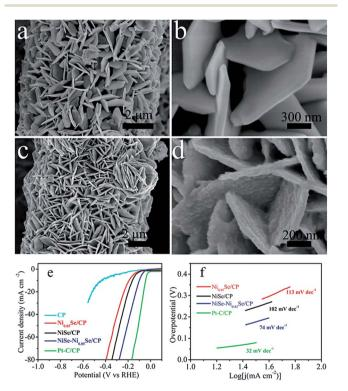
Fig. 8 (a and b) SEM image of NiO/CP. (c and d) SEM image of NiSe–Ni $_{0.85}$ Se/CP. (e and f) HER LSVs and the Tafel slope of NiSe–Ni $_{0.85}$ Se/CP in comparison with other studied catalysts in 1 M KOH. Reproduced with permission from ref. 74 (Copyright 2018 Wiley Publications).
