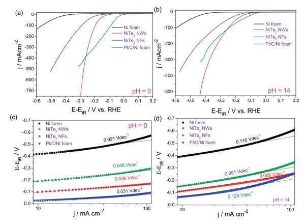
Fig. 12 (a and b) HER LSVs of NiTe<sub>2</sub> NWs, NiTe<sub>2</sub> NFs, Ni foam and Pt/C-Ni foam in 0.5 M H<sub>2</sub>SO<sub>4</sub> and 1.0 M KOH, respectively (sweep rate - 5 mV s<sup>-1</sup>). (c and d) Tafel plots of the same. Reproduced with permission from ref. 91 (Copyright 2018 American Chemical Society).
