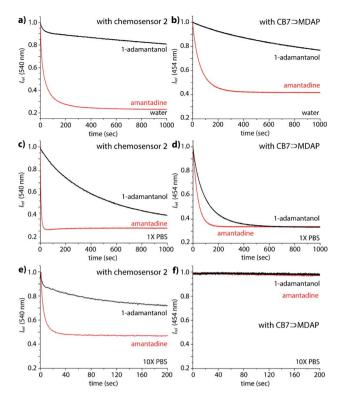
Fig. 5 Fluorescence-based kinetic traces at 540 nm of 1.2  $\mu$ M **2** and 2.09  $\mu$ M amantadine (red) or 1-adamantanol (black) in (a) water, (c) 1× PBS and (e) 10× PBS at 25 °C,  $\lambda_{\rm ex}=350$  nm; fluorescence-based kinetic traces at 454 nm of 1.8  $\mu$ M MDAP, 1.2  $\mu$ M CB7 and 2.09  $\mu$ M amantadine (red) or 1-adamantanol in (b) water, (d) 1× PBS and (f) 10× PBS at 25 °C,  $\lambda_{\rm ex}=339$  nm.
