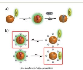
Fig. 1 (a) Schematic representation of analyte-induced conformational changes of CB7-dye conjugates that can be detected by emission spectroscopy; (b) schematic representation of the equilibrium between free- and bound-formation of CB7-dye with/without linker in the presence of a high concentration of interferents.
