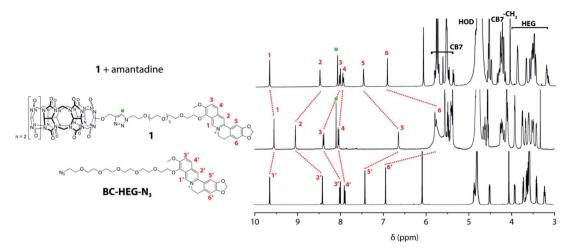
Fig. 3 Overlay of  ${}^{1}$ H NMR (500 MHz, D<sub>2</sub>O) spectra of BC-HEG-N<sub>3</sub> (bottom), chemosensor **1** (middle) and chemosensor **1** with one equivalent of amantadine (top).
