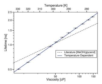
Fig. 4  $\log-\log$  plot of the temperature dependent fluorescence lifetime of BODIPY-C10 in the ionic liquid  $[C_4C_1im][NTf_2]$  against the viscosity at the corresponding temperature, taken from ref. 28. The blue line is the best fit to this data (eqn (3)). The dashed black line is the fit to values derived from the literature methanol/glycerol calibration.<sup>12</sup>
