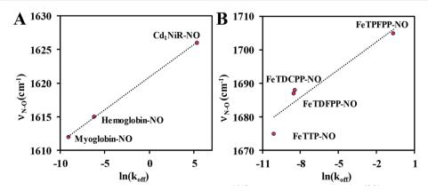
Fig. 2 Correlation between N-O stretching frequency<sup>16-18</sup> and rate of NO dissociation:<sup>19-21</sup> (A) in six-coordinate heme nitrosyls in enzyme systems; (B) in synthetic Fe-porphyrin nitrosyl complexes, TTP ( $\rho$ -tolyl), TDFPP (2,6-difluorophenyl), TDCPP (2,6-dichlorophenyl), TPFPP (pentafluorophenyl).
