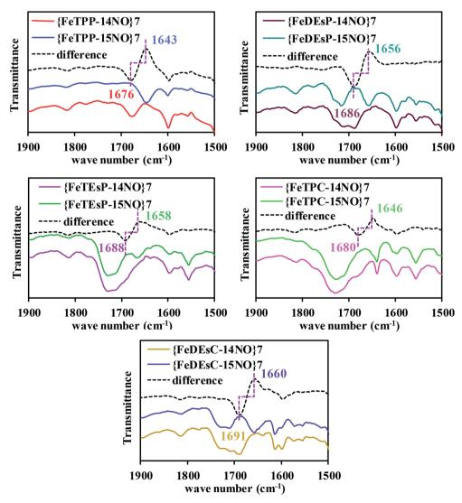
Fig. 6 FTIR data of the (FeNO)<sup>7</sup> adducts in dichloromethane at room temperature.
