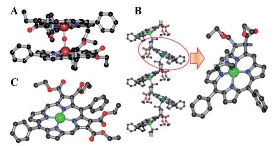
Fig. 4 Molecular structures of the crystals of (A) a μ-oxo dimer of FeDEsP; (B) ZnDEsC, and (C) ZnTEsP. Color code: C, black; Fe, brownish-red; Zn, green; N, blue; O, red. Hydrogen atoms are omitted for clarity.
