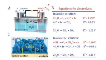
Fig. 1 Principles of water splitting devices. (A) Schematic illustration of the water splitting cell. (B) The reactions at the anode and cathode under the acidic and alkaline conditions of water splitting. (C) The freestanding oxygen evolution reaction electrode prepared *via* electrodeposition has close contact between the catalyst and substrate, avoiding the use of conducting carbon and polymeric binder.
