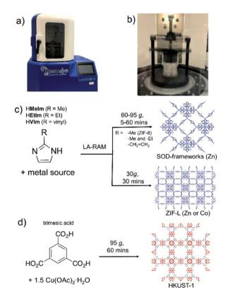
Fig. 1 Herein employed LabRam resonant acoustic mixer: (a) exterior and (b) interior shown during operation. Schematic illustration of herein developed MOF syntheses using RAM: (c) ZIF-8, mixed-ligand SOD-Zn(Melm)(Etlm) and ZIF-L (Zn and Co variants) and (d) copperbased HKUST-1
