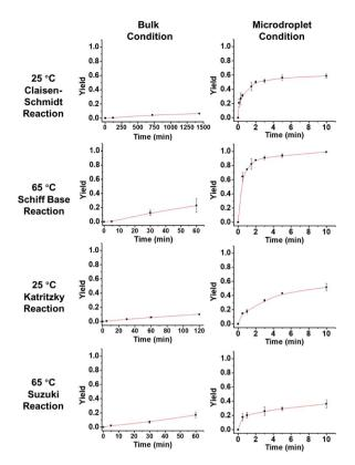
Fig. 3 Yield vs. time behavior of the four reactions under consideration. In order to obtain measurable kinetics curves in bulk, 20 equivalent KOH had to be used as opposed to 2 equiv. in droplets.
