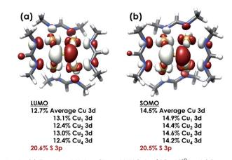
Fig. 5 (a) Restricted Kohn–Sham LUMO for [4Cu:1S]<sup>0</sup> and (b) quasi-restricted (QRO)<sup>33</sup> SOMO for [4Cu:1S]<sup>1—</sup>. Both MOs were calculated for truncated models using the B3LYP hybrid density functional with the CP(PPP) basis set on Cu and the scalar-relativistically recontracted ZORA-def2-TZVP(-f) basis set on all other atoms. Orbitals are plotted at an isovalue of 0.03 au.
