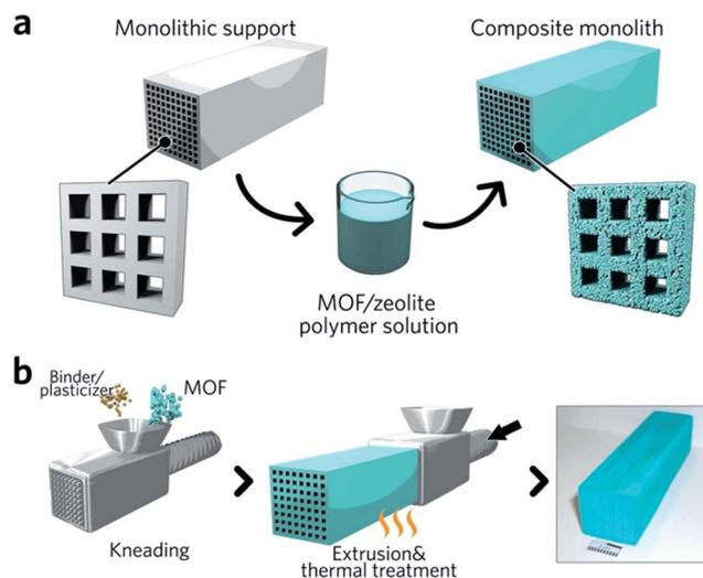
**Fig. 3** Fabrication of composite monolithic MOFs. (a) Wash coating to deposit MOFs on monolithic supports. (b) Extrusion approach for the fabrication of monolithic MOFs, with an optical photo of the resulting MOF monolith. Reproduced from ref. 67 with permission from the John Wiley & Sons, copyright 2010.
