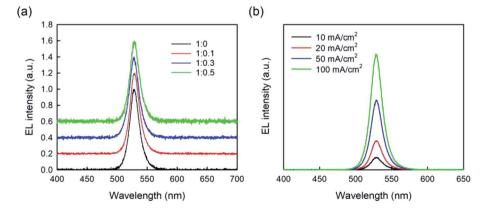
Fig. 8 (a) Normalized EL spectra of the PeLEDs with PEDOT:PSS HTLs doped with different GO amount tested at the current density of 50 mA  $cm^{-2}$ . (b) EL spectra for the PeLED with the optimal PEDOT:PSS:GO (1 : 0.3) HTL tested by using different current densities.
