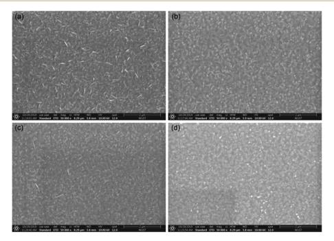
Fig. 4 SEM images of the  $CH_3NH_3PbBr_3$  films on the GO-doped composite films with different GO concentration of (a) 1:0, (b) 1:0.1, (c) 1:0.3, (d) 1:0.5.
