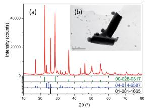
Fig. 3 (a) XRD pattern of anhydrous niobium oxide and the identified patterns. In the inset (b), a TEM image of the crystalline particles is shown (scale bar of  $0.5~\mu m$ ).
