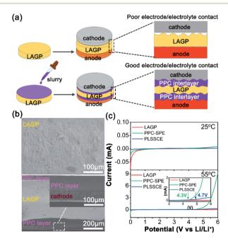
Fig. 1 (a) Schematic of the batteries design with pure LAGP electrolyte and PLSSCE. (b) SEM image of the LAGP surface (top) and the crosssection image of the PLSSCE/LiFePO<sub>4</sub> interface (below, with a partially enlarged view of the dotted box) (c) LSV curves obtained for the pure LAGP pellet, PPC-SPE and PLSSCE at 25 °C and 55 °C
