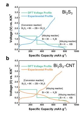
Fig. 3 Comparison of experimental charge–discharge curves of (a) the  $Bi_2S_3$  anode and (b)  $Bi_2S_3$ -CNT anode in the voltage range 0.01–3.0 V at 10 mA  $\rm g^{-1}$  and predicted voltage curves using first-principles calculation.
