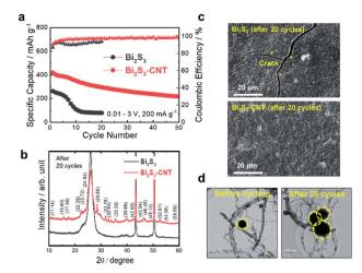
Fig. 5 (a) Cycle life test of  $Bi_2S_3$  and  $Bi_2S_3$ -CNT electrodes in the voltage range 0.01–3.0 V at 200 mA  $g^{-1}$ . (b) XRD patterns (c) SEM images of cycled  $Bi_2S_3$  and  $Bi_2S_3$ -CNT electrode after 20 cycles. (d) TEM images of cycled  $Bi_2S_3$ -CNT particles after 20 cycles.
