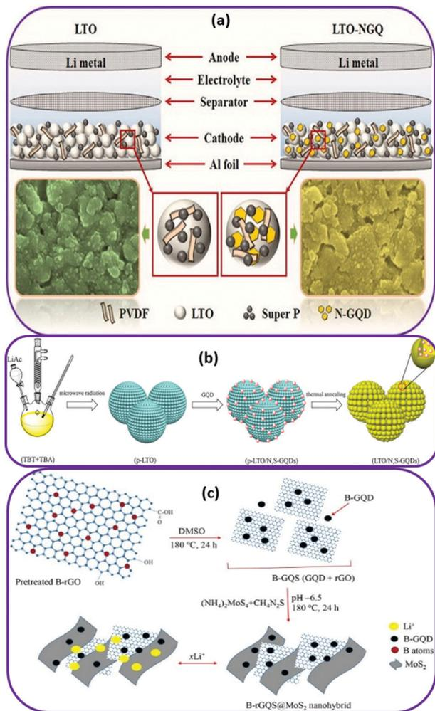
**Fig. 9** (a) Schematic of LTO/NGQD and pristine LTO as anode materials. Reprinted with permission from ref. 89. Copyright 2019, Elsevier. (b) Procedure for the synthesis of LTO/N,S-GQDs. Reprinted with permission from ref. 90. Copyright 2015, Elsevier. (c) Schematic illustration of preparation of BGQS/MoS<sub>2</sub> nano hybrids and the application for Li<sup>+</sup> ion intercalation/deintercalation. Reprinted with permission from ref. 92. Copyright 2019, Frontiers.
