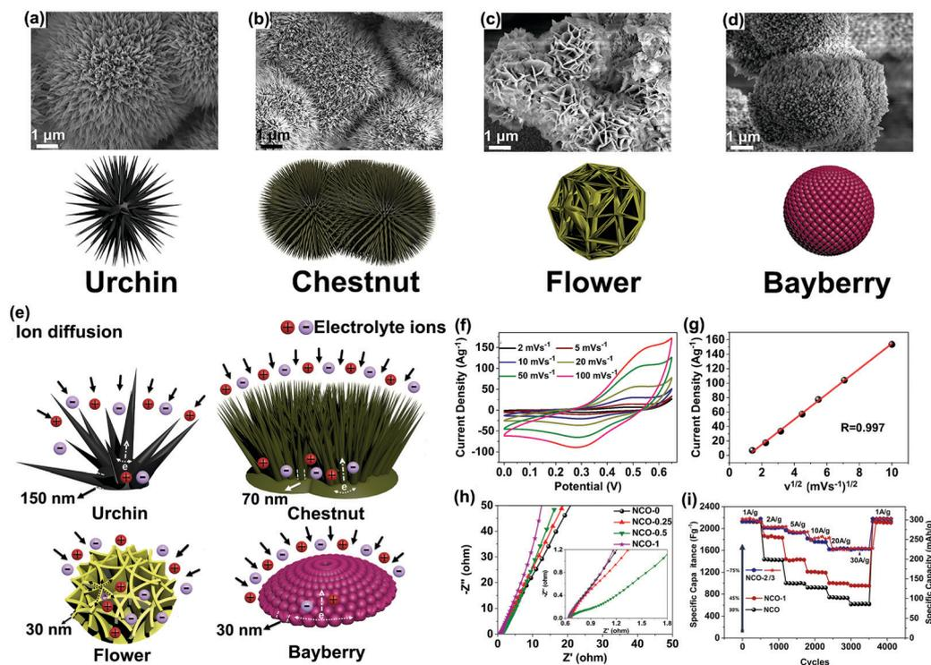
Fig. 7 (a–d) The CDs/ $\text{NiCo}_2\text{O}_4$  composites with different morphologies. (e) Simulation of ion diffusion on the material surfaces. (f) CV curves and (g) the relationship between current density of the optimal sample (NCO-0.5). (h) Nyquist impedance plots at the open-circuit potential. (i) Cycling and rate performances at various current densities. Reproduced with permission from ref. 27. Copyright 2016, Wiley-VCH.
