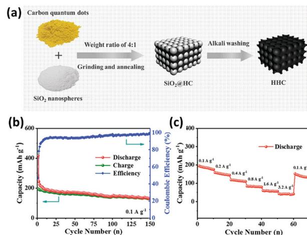
**Fig. 12** (a) The designed illustration of honeycomb-like hard carbon (HHC); (b) cycling performance at 0.1 A g<sup>-1</sup>; (c) rate capability at various current densities. Reprinted with permission from ref. 119. Copyright 2019, Elsevier.
