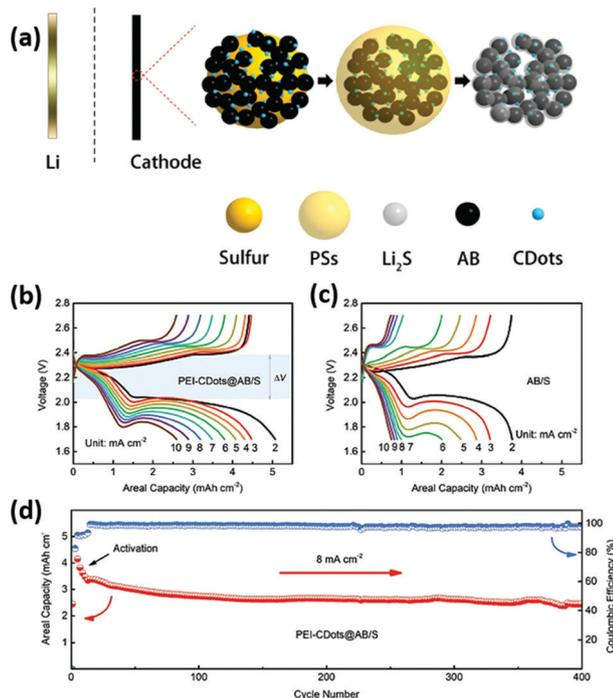
**Fig. 14** (a) Illustrations of the PEI-CDots-modified cathode composite at different charge–discharge stages. The charge/discharge profiles of (b) the PEI-CDots@AB/S cathode and (c) the AB/S cathode between 1.7 and 2.7 V. (d) The long-term cycling performance of the PEI-CDots@AB/S cathode with a sulfur loading of 6.6 mg, activated from 2 to 8 mA cm<sup>-2</sup> with 1 mA cm<sup>-2</sup> interval between each cycle. Reprinted with permission from ref. 128. Copyright 2018, Wiley-VCH.
