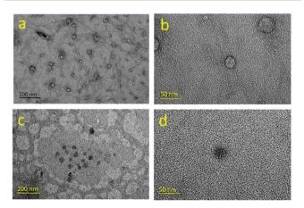
Fig. 5 TEM images for poly(A2-alt-B1)<sub>10</sub> (a, b) and poly(A2-alt-B1)<sub>50</sub> (c, d). 1 wt% samples in deionized water were dried on copper grids for TEM imaging.
