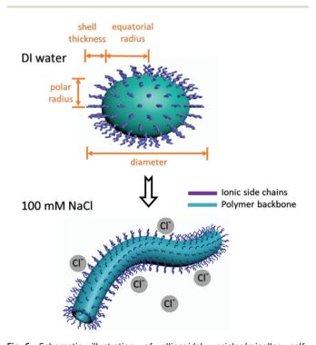
Fig. 6 Schematic illustration of ellipsoidal vesicles/micelles selfassembled from 10-mers and 50-mers in deionized (DI) water (upper panel where the core and the shell consisted of hydrophobic and hydrophilic segments, respectively. Both the 10-mer and the 50-mers selfassembled into cylinders in 100 mM aqueous NaCl (lower panel); both assemblies transformed into cylinders in 100 mM NaCl solution.
