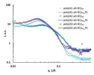
Fig. 3 SAXS data for poly(As-alt-B1)<sub>10</sub> assemblies (symbols) and fits to a core-shell ellipsoid model with a hard sphere structure factor (curves).
