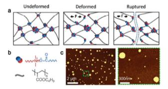
Fig. 16 (a) Schematic evolution of a non-covalent network under stretching, (b) electrostatic interactions and the chain backbone, and (c) AFM phase diagram of ionic polymethacrylate. Reproduced from ref. 108 with permission from the Royal Society of Chemistry, copyright 2018.
