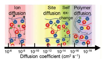
Fig. 5 Intrinsic and extrinsic diffusion processes within ionic polymer materials ranked according to their diffusion coefficients. Reprinted with permission from ref. 56. Copyright 2017, American Chemical Society.
