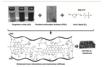
Fig. 22 Biobased membrane with enhanced ionic interactions for the design of artificial muscles. Reprinted with permission from ref. 178. Copyright 2013, John Wiley & Sons, Inc.
