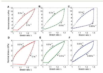
Fig. 4 Long et al. model fitting (dashed lines) with loading-unloading cycles (solid lines). Two loading rates are presented:  $0.3 \text{ s}^{-1}$  (A-C) and  $0.01 \text{ s}^{-1}$  (D-F). Unloading rate varies from  $0.1 \text{ s}^{-1}$  (A and D) to  $0.001 \text{ s}^{-1}$ (C and F). Reprinted with permission from ref. 38. Copyright 2014, American Chemical Society.
