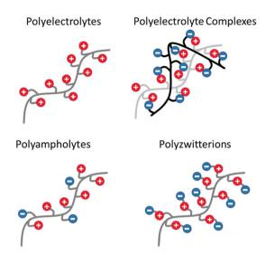
Fig. 12 Schematic representation of polyelectrolytes, polyelectrolyte complexes (association of oppositely charged polyelectrolytes), polyampholytes (polyelectrolytes bearing both cationic and anionic charges) and polyzwitterions (polyampholytes with the same amount of cationic and anionic functions on a repetitive unit).
