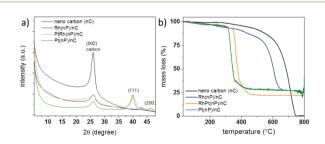
Fig. 1 (a) XRD patterns ( $CuK\alpha$ ) of the three composite materials Rh(nP)/nC (blue trace), PtRh(nP)/nC (orange trace), and Pt(nP)/nC (green trace) in comparison to the carbon starting material (nC, black trace). (b) Thermogravimetric analysis (TGA) of the three composite materials and the starting carbon material between 50–800 °C under synthetic air (80%  $N_2$ , 20%  $O_2$ ) with a heating ramp of 10 °C min<sup>-1</sup>.
