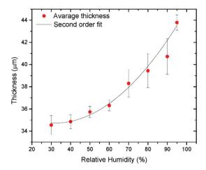
Fig. 7 Multilayered GO film thickness measured directly using ESEM as a function of humidity.<sup>129</sup>
