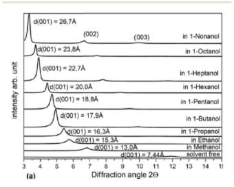
Fig. 14 XRD patterns recorded from Hummers GO in liquid alcohols. Reproduced from ref. 69 with permission from RSC, temperature/ pressure conditions, which makes higher alcohols attractive solvents for the preparation of pillared structures. It has also strong implications to the properties of multilayered GO membranes discussed in the next
