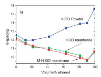
**Fig. 17** Interlayer distance, *d*(001), measured at 300 K for GO membranes in liquid water–ethanol binary solvents: (a) H-GO and M-H-GO membranes compared to H-GO. The M-H-GO membrane was produced in the same group which reported selective water pervaporation for water–ethanol binary mixtures.<sup>23</sup> Reproduced from ref. 224 with permission of RSC.
