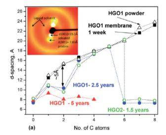
Fig. 19 Interlayer distance (d(001)) for Hummers GtO powder ( $\Delta$ ) and membranes immersed in liquid alcohols: freshly prepared (1 week) sample ( $\blacksquare$ ), sample stored in air for 1.5 years, ( $\bigcirc$ ) for 2.5 years ( $\bigcirc$ ), and sample stored in air for 5 years ( $\triangle$ ). The inset shows the 2D XRD image ( $\lambda$  = 0.30996 Å) recorded of the Hummers GO membrane in 1-pentanol after 7.5 hours of immersion.
