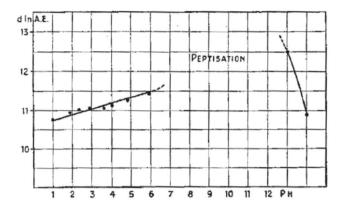
Fig. 2 Inter-layer distance value provided by d(001) from XRD experiments as a function of pH.83 Graphite oxide spontaneously disperses into graphene oxide for the interval of pH marked as "peptisation.
