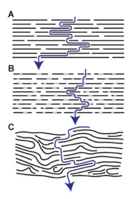
Fig. 16 Possible water-transport mechanisms through GO laminates. (A) Layer-by-layer water transport in which water flows strictly between the individual GO sheets. (B) Layer-by-layer transport, mediated by pinhole defects, in which the effective path length is significantly reduced by the pinhole defects. (C) Combination of layer-by-layer transport and transport mediated by voids and imperfect sheet stacking. Reproduced from ref. 239.
