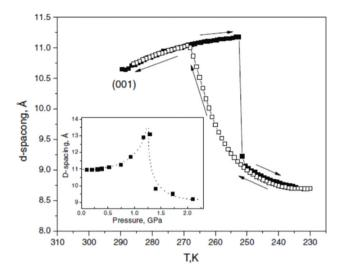
Fig. 9 Temperature dependence of the d(001) of Brodie graphite oxide immersed in liquid water. <sup>153</sup> The inset shows the pressure dependence of d(001) of GO/H<sub>2</sub>O. <sup>111</sup> Solidification of liquid water (at low temperature or high pressure) results in sharp downturn of d(001) due to partial withdrawal of water from the GO lattice.
