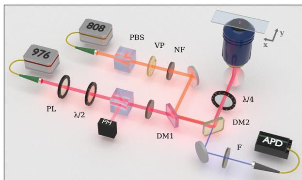
**Fig. 1** Schematic of the confocal microscope system, where PBS is a polarising beam splitter, VP a vortex plate, NF a neutral density filter, PL is a polariser,  $\lambda/2$  a half-wave plate, PM a power meter, DM1 and DM2 respectively a long-pass and short-pass dichroic mirror,  $\lambda/4$  a quarter-wave plate, F a blue narrow-band filter, and APD an avalanche photodiode.
