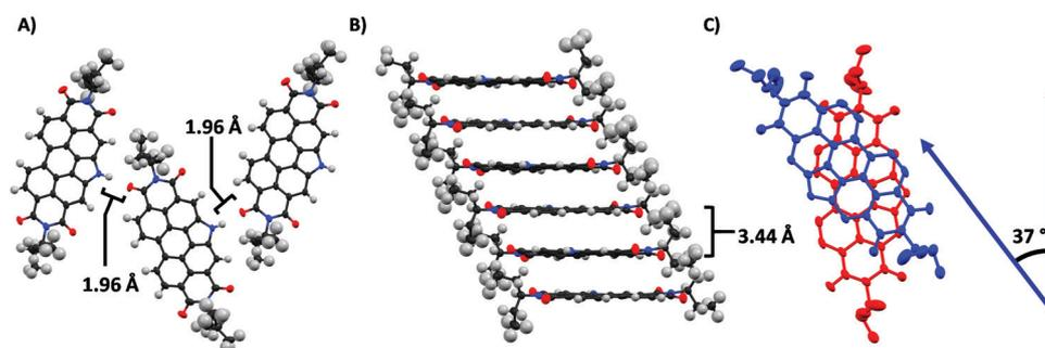
Fig. 8 Structural of PDIN-H highlighting: (A) hydrogen bonding between the NH and C=O functional groups, (B)  $\pi$ - $\pi$  stacking motif, and (C) the offset and dihedral angle between two  $\pi$ -stacked molecules. In (A) and (B) C, H, N, and O atoms are shown as grey, white, blue, and red, respectively. In (C), H atoms have been omitted for clarity and one molecule of PDIN-H is represented in blue and another in red.
