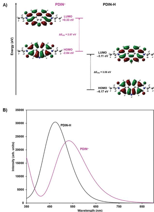
Fig. 3 (A) Schematic molecular orbital (MO) correlation diagram for PDIN<sup>-</sup> (left, purple) and PDIN-H (right, black) as determined at the M06/6-31G(d,p) level of theory. (B) Simulated absorption spectra of PDIN<sup>-</sup> (purple) and PDIN-H (black) derived from TDDFT calculations at the M06/6-31G(d,p) level of theory.
